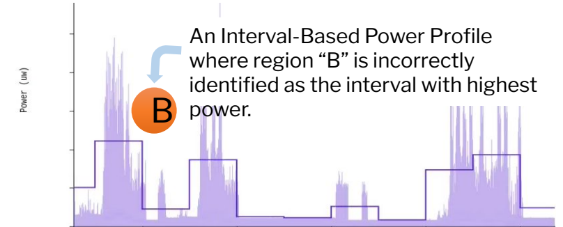
Figure 1: Time Interval 'B' with highest average power \Delta = \text{Window} = (100 * \text{FastestClockPeriod})
